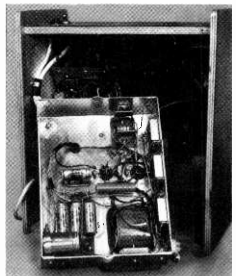
Fig. 6. Layout of oscillator and power unit chassis. (Connections to the X and Y amplifiers and the bridge circuit are made via a multi-way connection block on top of the chassis)
